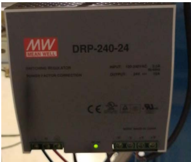
Figura 5.1 (power supply 24 V 10 A)
